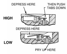
Be bent, extruded from being forced into the casting seat or possibly broken off in the casting. If either mixture screw is damaged, be sure to inspect the condition of the casting. If the adjustment seats are damaged, a new body casting is required.
