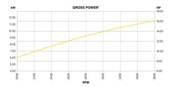
All power levels are stated in gross kilowatts per SAE J1940 as rated by Briggs & Stratton.
