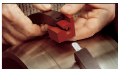
Stage 2: Align joint in moulded jig.
